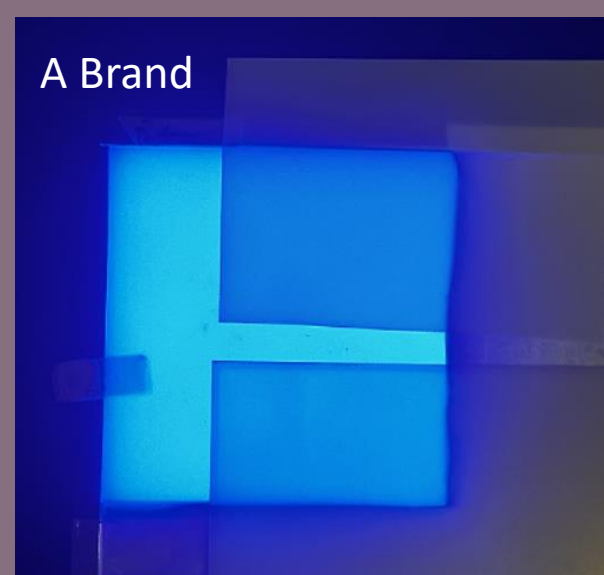
Degradation of QD in the edge region of film
